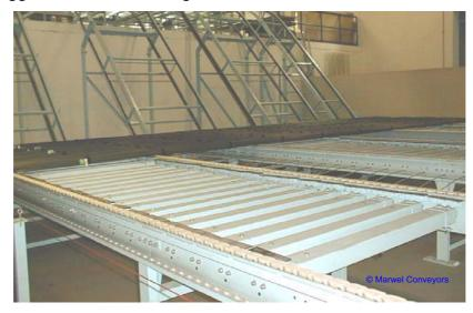
The above photograph shows a multi-chain accumulating conveyor used for storing long bundles of tubes. Also shown is a multi chain elevator used for transferring tubes from one level to a higher level.
