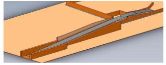
The second type is based on a rubber belt with a special surface we have called "boat grip" This unique belt surface gives a high coefficient of friction. It is especially effective when operating under wet conditions against the advanced materials used in the construction of modern kayaks. These conveyors are available up to 2.1 metres wide.
