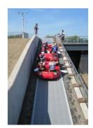
The first type of conveyor is based on a perforated modular plastic belt They can be supplied in a wide range of widths & colours.
