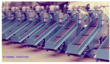
Marwel Conveyors manufacture a range of conveyors suitable for handling hot forgings.
