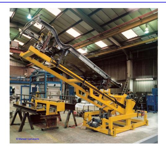
MARWEL CONVEYORS LTD CAN SUPPLY A RANGE OF UPENDERS AND DOWNENDERS TO SUIT A VARIETY OF PRODUCTS. EACH UNIT IS CUSTOM DESIGNED TO FIT INTO A MECHANICAL HANDLING SYSTEM.
