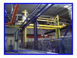
Transporters are widely used in the finishing industry for moving components between process tanks.
