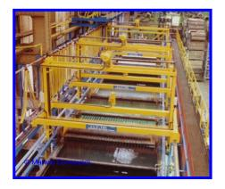
Transporters can be fitted with special grabs to handle the components directly, or where a variety of components need to be handled, the transporter can handle a standard flight bar, from which the components are
