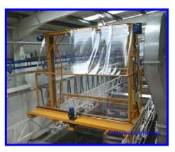
Transporters generally interface with other conveyor systems such as overhead conveyors or floor conveyors.
