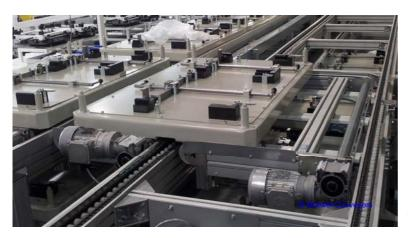
Typical are those used for moving pallets between conveyors.
