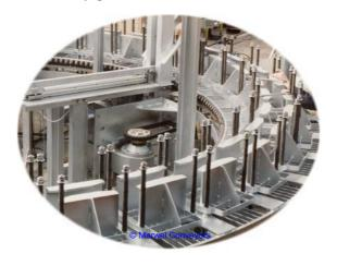
They typically have a series of load carrying platforms connected together to form a continuous chain or the platforms can be fixed to a carrying or towing chain.
