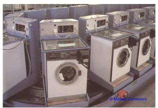
The platforms follow a fixed path in a continuous loop with or without changing height.
