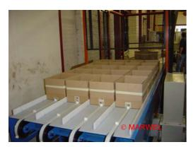
Belt Conveyors can consist of single belts or multiple belts with attachments as shown above.
